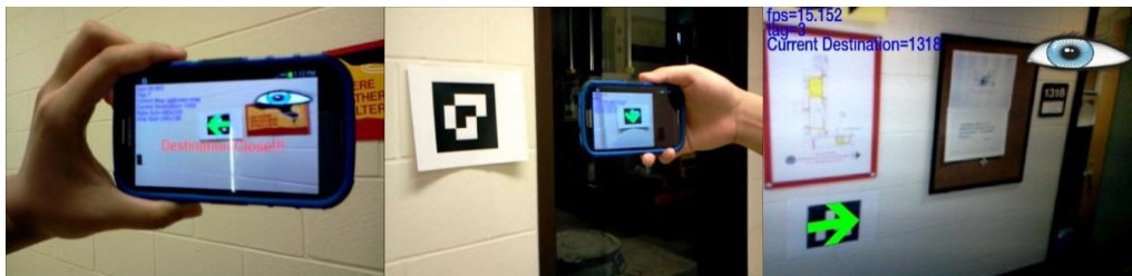
Figure 2 – Object identification and pose estimation for indoor inspection and maintenance
